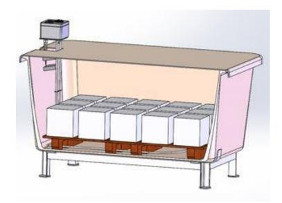
The outer vessel and the cover of the Climate-Controlled Chest are made of polyethylene.
