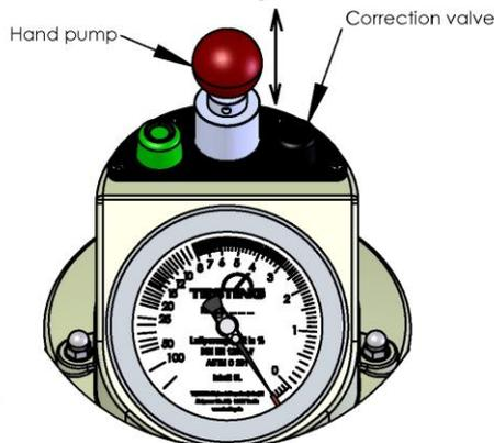
9. Operate the TEST valve. The pointer must now stand exactly over the zero. If the pointer is below the zero, push the red marker in the direction of zero. If the pointer is above the zero, move the marker in the other direction.
