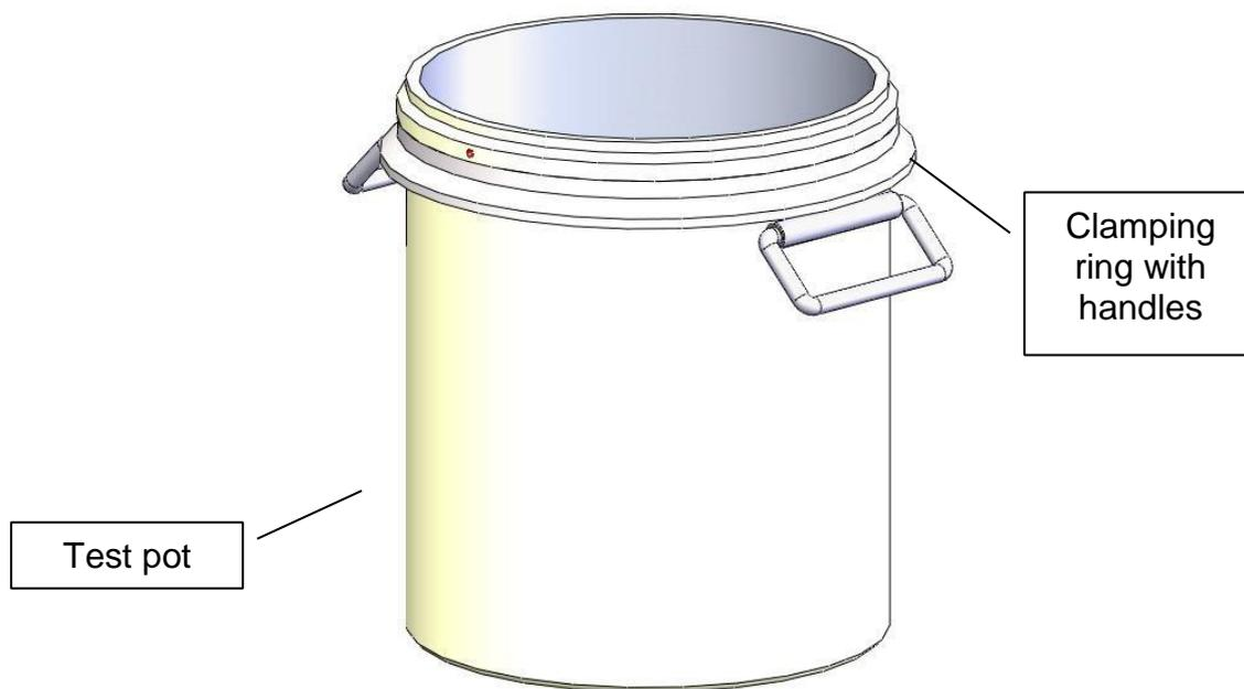
The outside of the air entrainment meters is an enclosure made of anodized cast aluminium. The upper part and the test pot are held together, air-tight, by quick-release latches. The water is filled in through the two ball shut-off valves, and air-pressure release takes place through these same valves.
