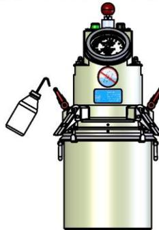
6. While the water is flowing constantly, tip the unit on its side and rotate it in circular motion until the water flows out of the right ball shut-off valve without bubbles.
