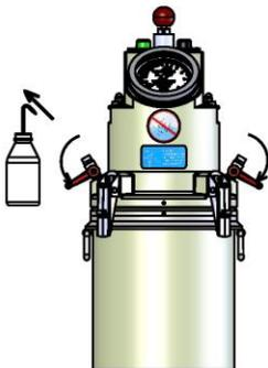
8. Use the hand pump to pump up the unit until the pointer has moved past the red marking. Then use the CORRECTION valve to adjust the pointer position, so that it is exactly over the red marking.
