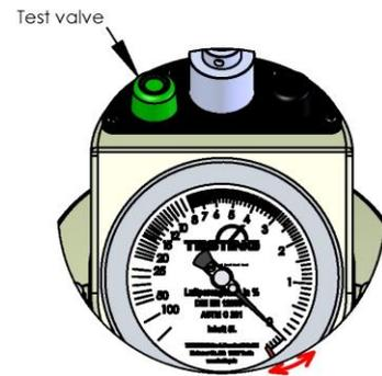
10. Screw down the threaded tube onto the left ball shut-off valve. Let the tube hang into a suitable graduated cylinder and open the ball shut-off valve. Operate the TEST valve and pump with the hand pump until 100ml (1-litre unit), 250ml (5-litre unit), or 400ml (8-litre unit) of water has flowed out. Then close the left ball shut-off valve.
