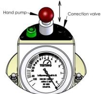
9. Operate the TEST valve. The pointer must now stand exactly over the zero. If the pointer is below the zero, push the red marker in the direction of zero. If the pointer is above the zero, move the marker in the other direction.
