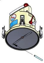
3. Place the upper part down onto the test pot, and snap the quick-release latches downward. Make sure that the markings on the top and bottom parts are in line, and that the angles
