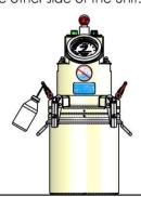
6. While the water is flowing constantly, tip the unit on its side and rotate it in circular motion until the water flows out of the right ball shut-off valve without
