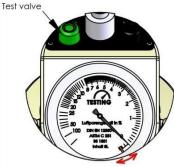
10. Screw down the threaded tube onto the left ball shut-off valve. Let the tube hang into a suitable graduated cylinder and open the ball shut-off valve. Operate the TEST valve and pump with the hand pump until 100ml (1-litre unit), 250ml (5-litre unit), or 400ml (8-litre unit) of water has flowed out. Then close the left ball shut-off valve.
