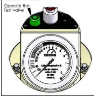
5. Open the shut-off valves and fill the vessel with a hose or a squeeze bottle. Fill until the water flows out constantly on the other side of the unit.
