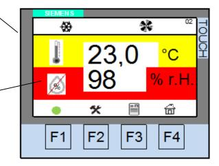
Yello field means: One of the two installed fans doesn't work Regulation is still ON
