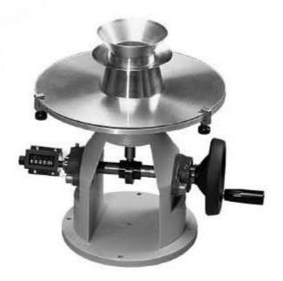
1.0223E Design with stainless steel table top based on DIN EN 1015-3
